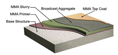
T-18 is applied using a single application slurry method. It is easy to handle and does not require any specialized installation equipment.
